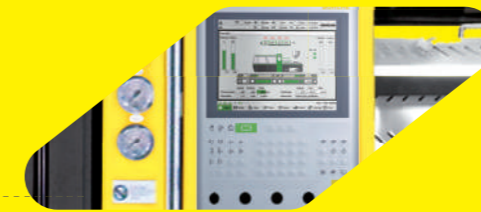
Automatic control Austria made KEBA controller model 2880
